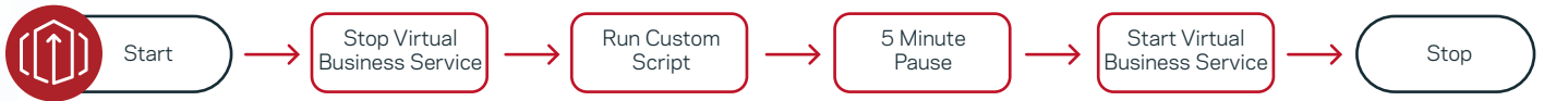
Figure 8. An example of the resiliency plan for automated failover of an IT business service.
