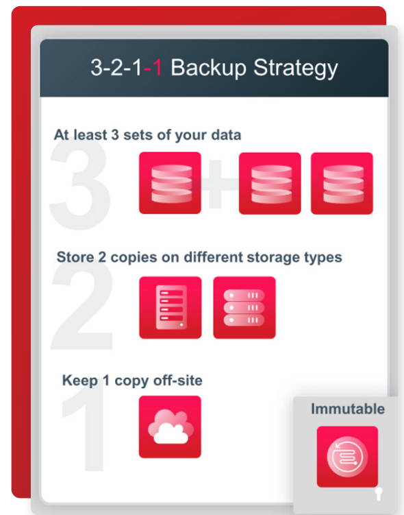
Figure 1. A best practice is to save at least three copies of your data on at least two types of storage with one off-site and one on immutable/WORM storage.
