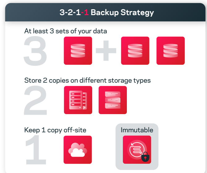
Figure 2. Keep three copies of data on two types of storage, with one copy off-site and one on immutable storage.
