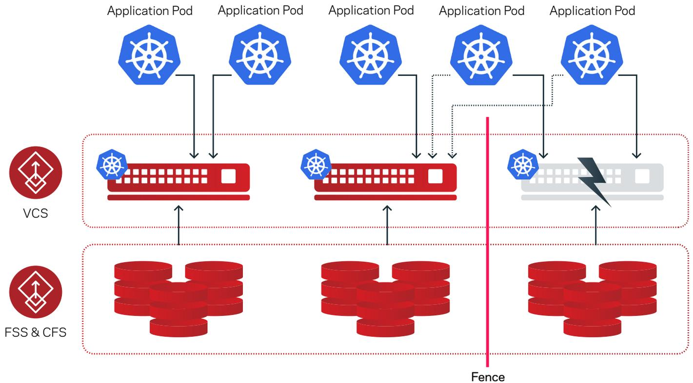
Figure 8. I/O fencing in Kubernetes using InfoScale
