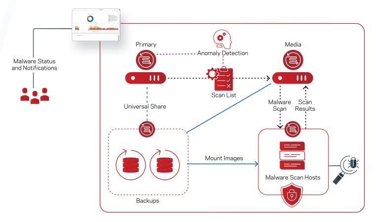
An on-demand scan model in the NetBackup WebUI is focused on periodic inspection of images, with the option of enabling automatic scanning for images with high Anomaly Detection scores. Focus your on-demand scans against the high-risk hosts—hosts interfacing with the public internet, Internet-of-Things (IoT) devices, and other edge machines.
