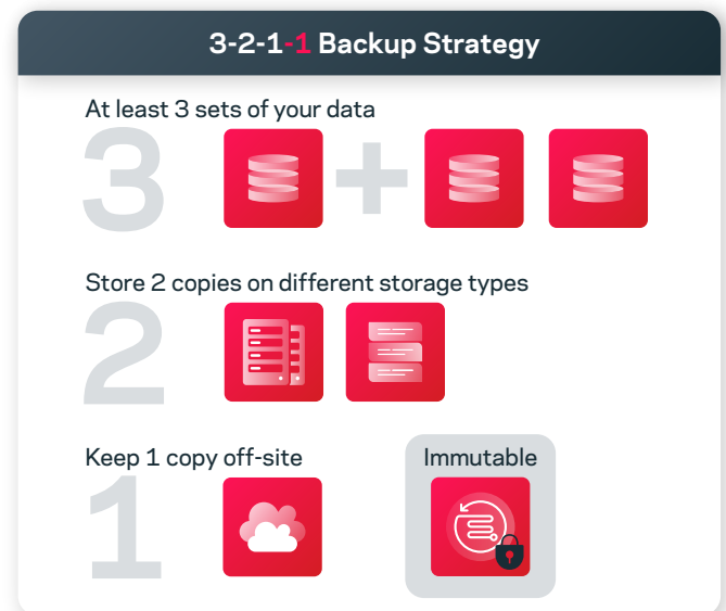
Figure 2. Keep three copies of data on two types of storage, with one copy off-site and one on immutable storage.
